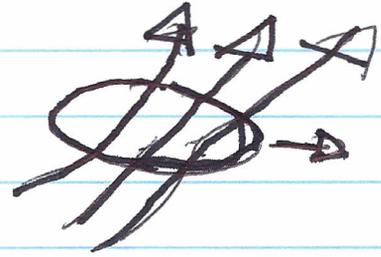
⇒ MHD is two interpenetrating 'fluids' of  $\underline{v}$  and  $\underline{B}$  frozen into each other
